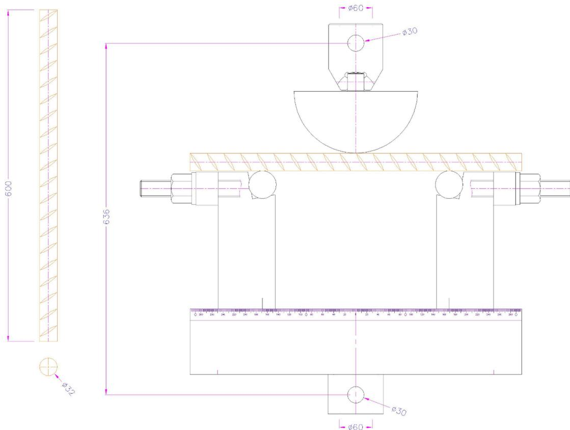
Schematic Comment: For this fixture, the space is adjustable between the contact supports that hold the specimen
